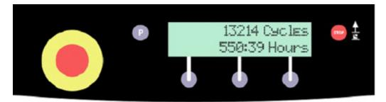
Upon entering the User Mode menu, a screen will appear showing your SK450 's life in mixing cycles and total hours. Press the program button to run through the different user menu's.
