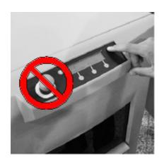
To interrupt the mixing program, press the stop button. Use the emergency stop only in case of calamity.
