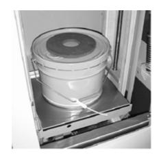
When the program finishes or is interrupted with the stop button, the SK450 will unclamp automatically.
