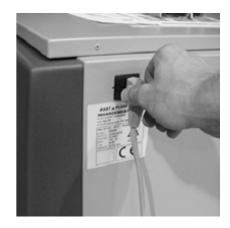
Connect the SK450 to the power mains before closing the door.
