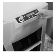
Choose correct program and press desired timing button. Clamping and mixing will now start.
