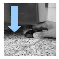
Lower the adjustable feet far enough to lift the machine off its wheels.
