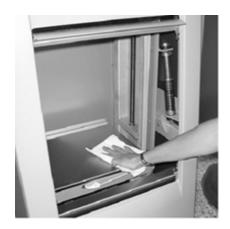
Remove all spilt paint from accessible parts (especially clamping plate spindles). Use diluted detergent only and Teflon spray only.
