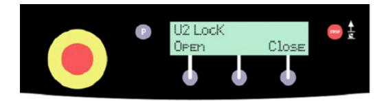
The U2 option is used to either lock or unlock the door manually. This may be necessary after a power failure or accidentally closing the door while the power is down.
