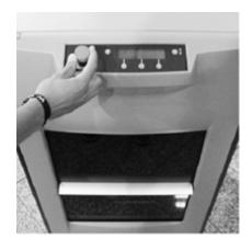
Turn the emergency stop clockwise to unlock: the screen displays the startup actions and 'ready' message.
