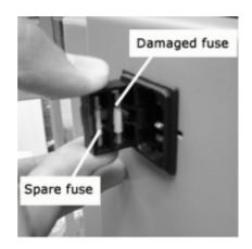
The inner fuse is the (damaged) one to replace, the outer is the spare to replace it with.
