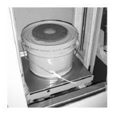
Place the container in the can table center, place filler disc and attach hook to container handle.
