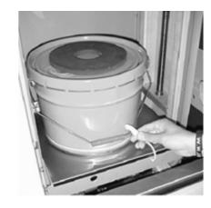
Use the hook to fixate the can handle. When mixing more than one can, use adhesive tape.
