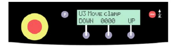
The U3 option is used to force the clamp plate to move either up or downwards. This may be necessary in case of the clamp plate jamming in its upper or lower position.
