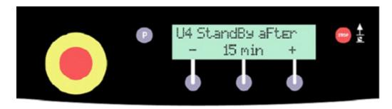
The U4 option is used to define the amount of time before entering standby modus.
