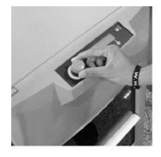
Ensure the emergency stop is unlocked (turn clockwise).
