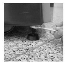
Lock all adjustable feet by tightening the their separate bolts.
