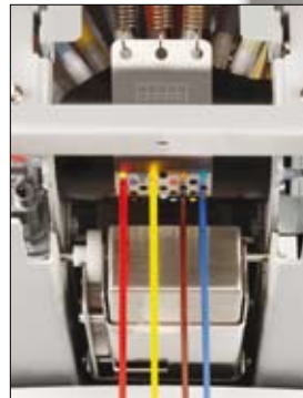
Simultaneous dispensing of four colours without leaving behind colorant residue.
