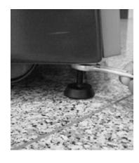
Lock all adjustable feet by tightening the their separate bolts.
