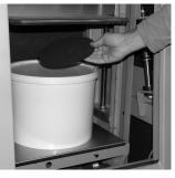
Place filler disc on lid to prevent displacement during operation.
