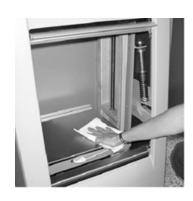
Remove all spilt paint from accessible parts (especially clamping plate spindles). Use diluted detergent only and Teflon spray only.
