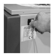
Connect the SK280 to the power mains before closing the door.
