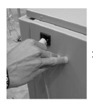
Remove mains connector and pull fuse tray outwards.
