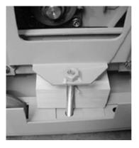
By removing the bolts, the frame lock's wooden block is released.
