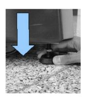
Lower the adjustable feet far enough to lift the machine off its wheels.
