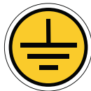
Central earthing point
