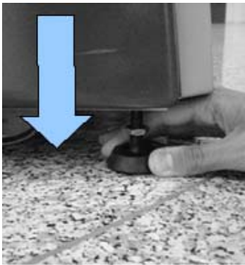
Lower the adjustable feet far enough to lift the machine off its wheels.
